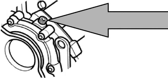
Lock the fuel pump pulley in its timed position with the pump timing marks aligned using **Component 1** as shown.
