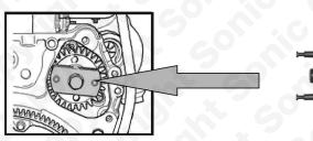
Component 3 - Water Pump Puller Component 3 is used to pull the water pump out as shown.
