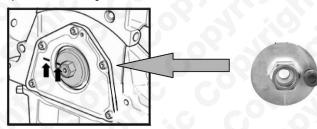
Component 2 - Water Pump Sprocket Puller Component 2 is used to remove the water pump pulley.
