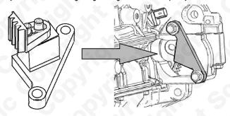
Balance Shaft Chain Tensioner Retaining Pin (2.5mm) (12).
