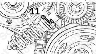
Camshaft Drive Chain Tensioner Plunger Resetting Tool and Holder (5&6).
