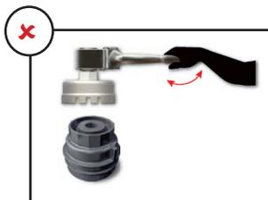
DO NOT use a ratchet wrench to remove an old filter cartridge. Use an extra socket for removal.
