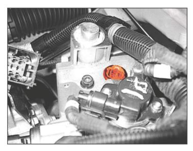
Undo the protection plug for the hydraulic unit selection lever locking tool.
