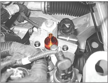
Install the tool to lock the selection lever inside the actuation hydraulic unit.
