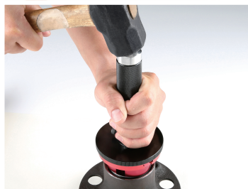
5) Tap the driver handle to force the race or seal into place.
