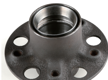
4) Place the race or seal in the mouth of the housing.
