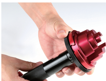
1) Loosen the screw, and then turn the dial to expand the jaws.
