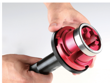
2) The face of the jaws seat against the race or seal.
