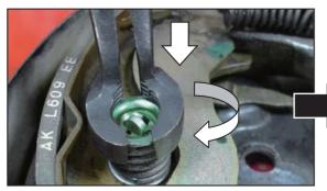
Hold the handle, clip the groove on the front ditch and rotate the tool.
