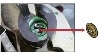
Remove/Install the spring washer smoothly.
