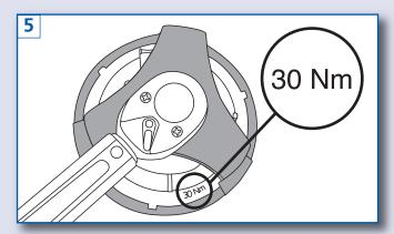
Tighten the fastening ring to 30Nm, then refit the housing to the vehicle and reconnect all fuel pipes and electrical connectors. Start the engine and check for leaks.
