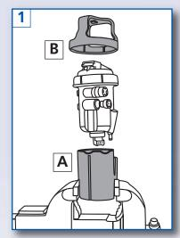
Clamp part 'A' into a vice. Remove fuel filter housing from vehicle, taking care to remove all pipes and all electrical connectors. Place the filter housing into part 'A' and locate part 'B' onto the top of the housing, aligning the six slots of the tool with the filter housing fastening ring.
