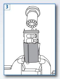
Extract the upper section of the filter housing and replace the fuel filter element (ADK82327) taking care not to touch the filter paper on the new element.
