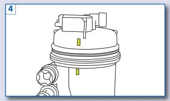
Replace the rubber seal between the two sections of the housing with the one supplied with the new filter. Refit the upper section to the housing by aligning the yellow/green markers.
