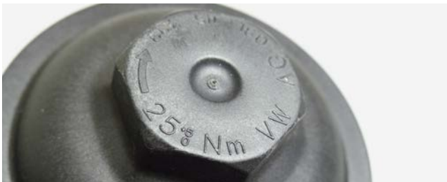
Figure 2: Torque specification on the housing cover
