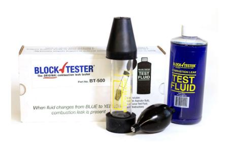
This Combustion Leak Test Fluid is designed to be used with our combustion leak test device (371-00) and aide in the detection of combustion gases released by cracked blocks, cracked heads, or failing head gaskets of the coolant system. This product may be used with any closed cooling system generator or internal combustion engine using a liquid coolant. This includes but may not be limited to gasoline, diesel, propane, natural gas or other alternative fuels.
