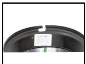
AIR LINE MUST BE ROUTED PROPERLY THROUGH THE NOTCH IN THE TOP MOUNT.
